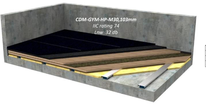
30mm GYM-ELAST-30 2xPW19 + DAMP5 CDM-GYMLAT-M30 16mm Acoustic Insulation
